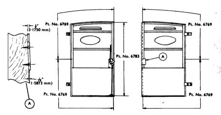
The sealing strips may be fitted to vehicles prior to the above engine number if required as follows:
